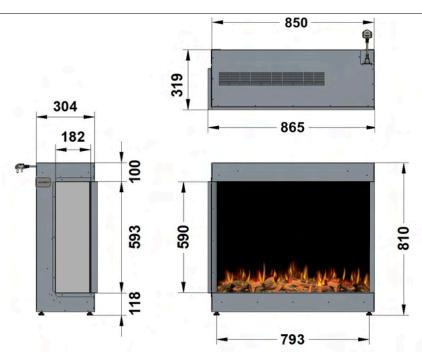
FRAME BUILD OUT DIMENSIONS (All dimensions are in millimetres)
